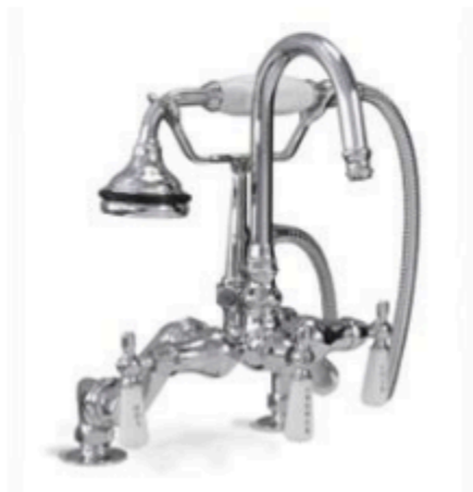
Edwardian Faucet with 2 " riser elbow ICS always uses center adjusters to open the 3 3/8" Edwardian faucet to a 7 inch spread for rough in.
