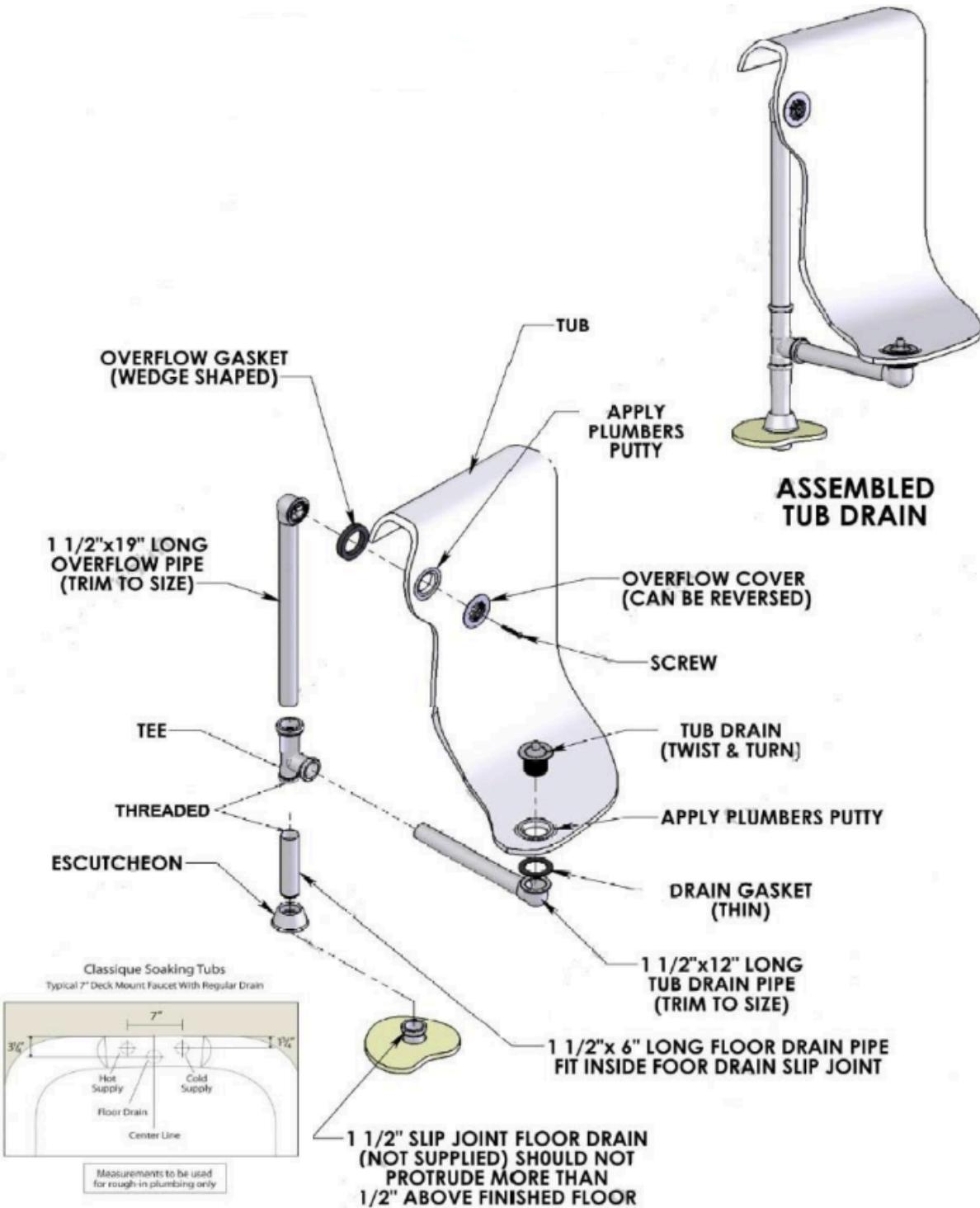
3 1/4 " for drain, 1 3/4 " for risers or 1.5 " from drain ctr to riser center
